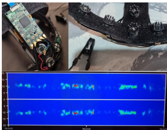
The effect of blinking and sampling the alpha signal by displaying it in the frequency domain.
